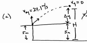
$$y_{1}^{2} = v_{-}y_{1}^{2} + 2\alpha_{1}\Delta_{1} = \lambda_{1} = \frac{-v_{0}y_{1}^{2}}{2\alpha_{1}} = \frac{-(24.1)^{2}}{2(-9.8)}$$
